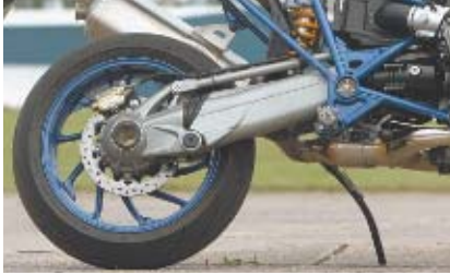
Paralever shaft drive is unnoticeable, as good as a chain
